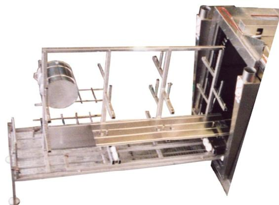
Our washing tunnel model "LIBRA" has been specifically designed for components coming from Roto and Flexo printing machines (inking trays, side covers, ink tanks, doctor blades, tools and other components).
